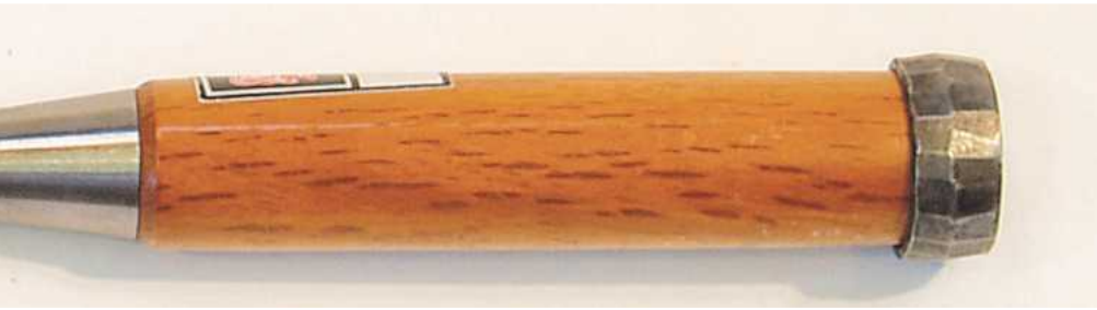
▲ Pic.7 A small mortise chisel for joints in small screens
